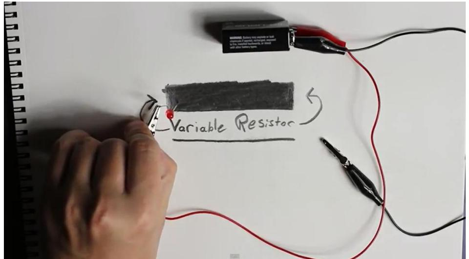
Place the extra alligator clip onto the end of the graphite bar and watch the LED light up. Slide this clip back and forth on the bar to watch the LED glow brighter!
